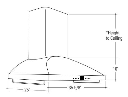
Note: Reference pub. no. 49-80095 for 36" ZV950 model, GE Monogram 36" Vent Hood Installation Instructions, before installing for current dimensional data.
